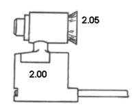
Insert Suction Cap Gasket (2.05) Completely Into Spiral (2.00).
