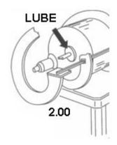
Slide Bowl (5.01) Back Onto Freezing Cylinder. Gently Snap Bowl Legs Into Place, Will õPopö.
