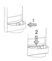
Insert Drip Tray (7.09) In Then Down. Insert Grate (7.10) Into Drip Tray (7.09). Plug Machine Power Cord (7.14) Into Wall.
